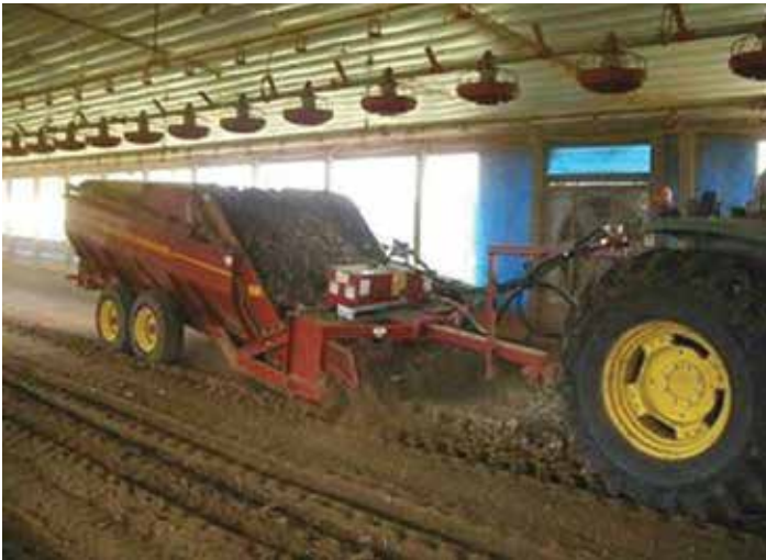
Figure 2. Machine used to scrape a layer of litter (manure and bedding) in the poultry house.
