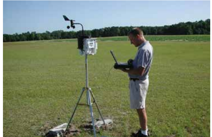
Figure 3. Tools and techniques available to estimate evapotranspiration and irrigation needs: (3.1) weather data may be simply downloaded from a small automated weather station to calculate reference evapotranspiration (ET o ) and (3.2) water loss in the reservoir of the atmometer mimics ET o .
